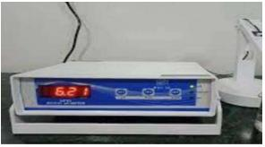
**2. Viscosity:** Viscosity was calculated at  $25\pm1^{\circ}$ C using a Brookfield viscometer (digital viscometer model). The rotation of the spindle was kept as 1 rpm. The solution equivalent of 10ml was taken into a volumetric flask (100ml) and diluted using methanol.
